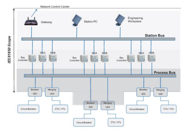
Figure 6: IEC 61850 Substation Bus Architecture
