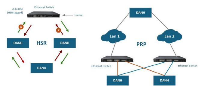
Figure 9: Comparison of High-Availability Seamless Redundancy (HSR) and Parallel Redundancy Protocol (PRP) in Network Communication
