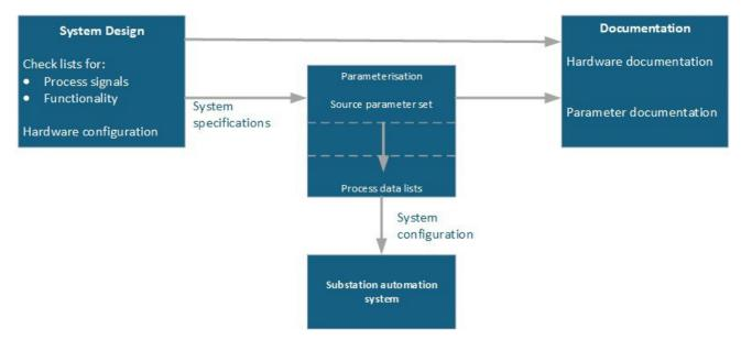
Figure 5: System Design, Parameterization, and Documentation Flow in Substation Automation (IEC 61850 Standard), Source: IEC 61850
