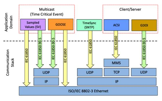
Figure 4: EC 61850-90-5 Protocol Stack Mapping to OSI Model Source: IEEE Access, Real-Time Control and Monitoring in Smart Grid, June 2017
