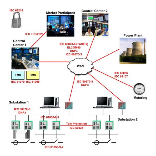
**Figure 3: Typical Communication Protocols Used in a Power System** Source: IEEE PES '09. Power & Energy Society General Meeting, Salman Mohagheghi 2009.
