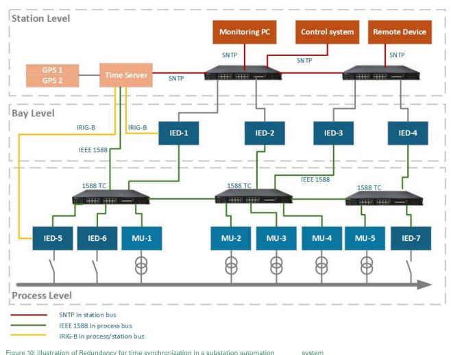
Figure 10: Illustration of Redundancy for time synchronization in a substation automation
