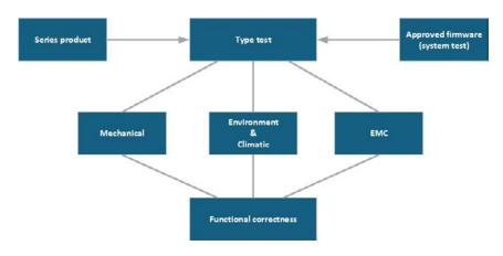
Figure 12: Testing Framework for Power Systems Automation (IEC 61850 Standard); Source: IEC 61850
