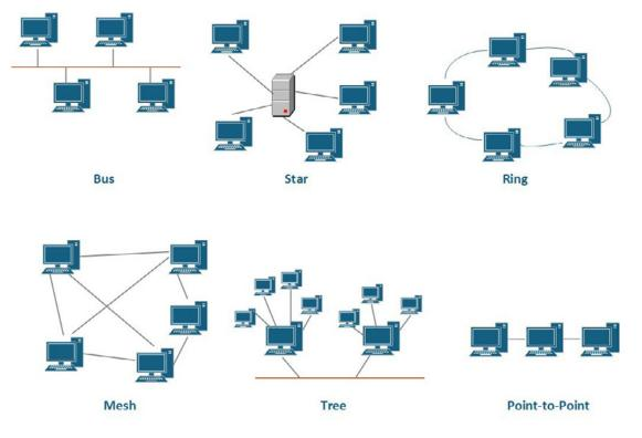
Figure 8: Common Network Topologies in Communication Systems
