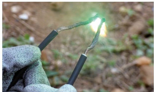
Figure 14: Example of an electric arc at the terminals of a 200 WP module under 1000 w/m 2 sunlight -
